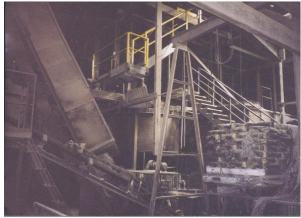
2011: Bldg 5 contained significant objects and systems for the transport of clay to the brick presses on the upper levels
